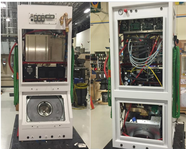
Figure 34. A single block, SSM based Mi6SSM (Tower) LINAC system primarily used for Security Screening. Temperature-Regulated Water Chiller and Operator Console come separately and not shown.
