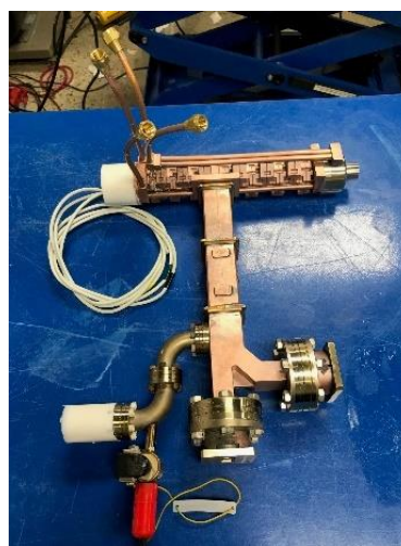
Figure 9. ABC-2.5-X-X-DI-T "Dual Input" designed for 2.5 MeV and dose rate up to 50 R/min@1 m from target.
