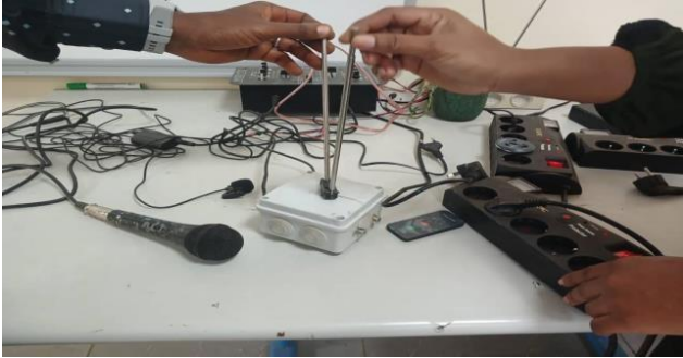
Figure 7. Adjusting the length of the feed antennas to improve range.
