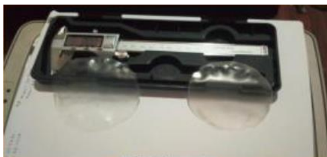
Figure 2. Film thickness measurement using digital micrometer.
