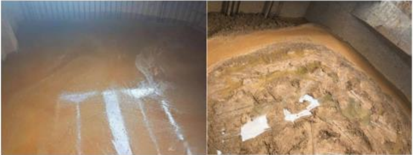
Figure 2. Liquefaction of Nickel Ore in the Cargo Hold.
