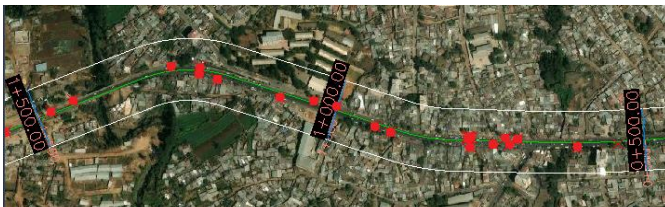
Figure 2. Road segmentation using Civil 3D.
