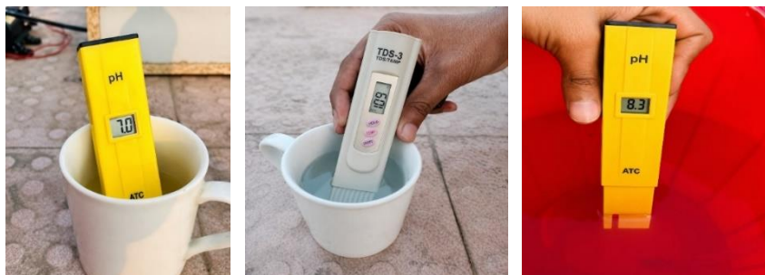
Figure 11. The figure shows three measurements: a pH of 7.0 and a TDS of 109 ppm for desalinated water, and a pH of 8.3 for brine water.
