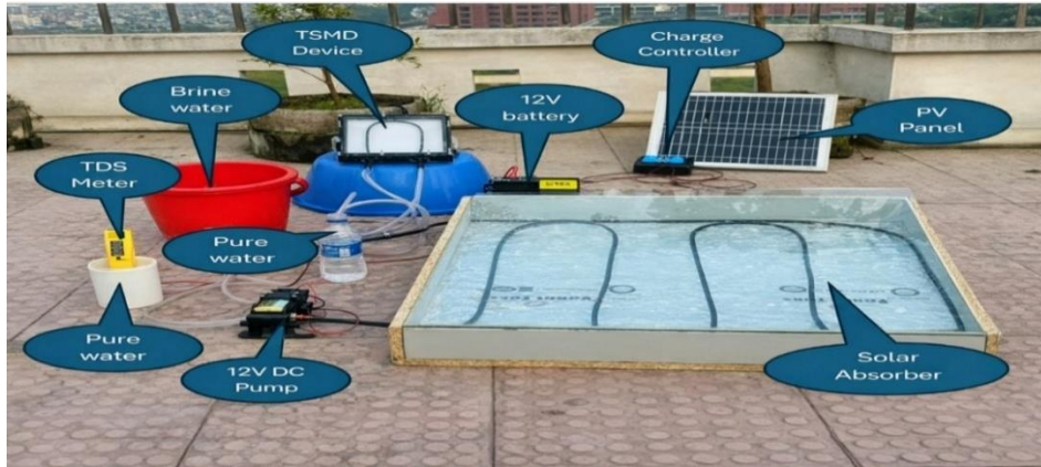
Figure 4. Hardware implementation of the complete TSMD system.
