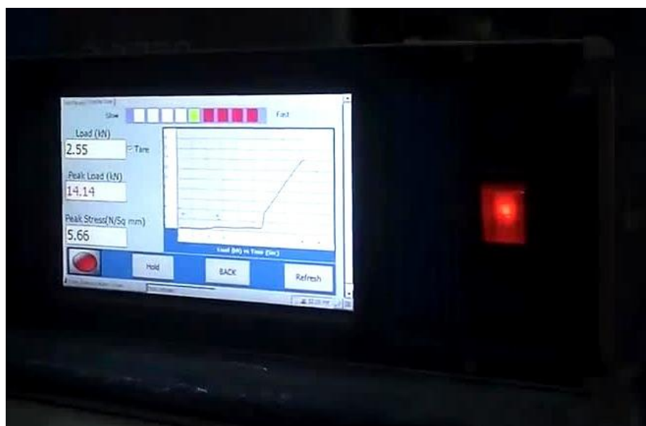
Figure 7. Four-point bending test arrangement and flexural UTM monitoring.
