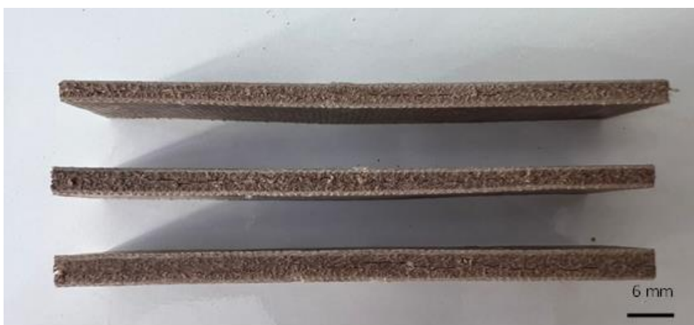
Figure 12. Hybrid composites aged at 60 °C showing cracks running along the entire side of the specimens.
