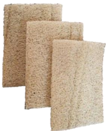
Figure 1. Sponge gourd blanket used to manufacture the sponge gourd and hybrid composites.
