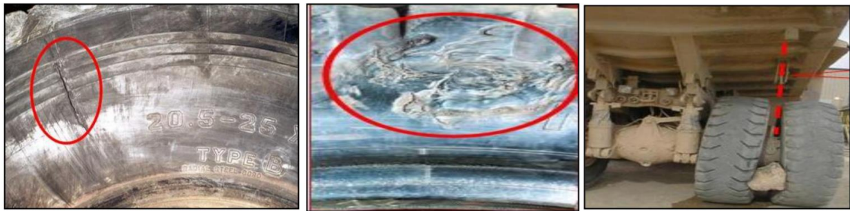
Figure 6. Haul Truck Tyre Sidewall Cut.
