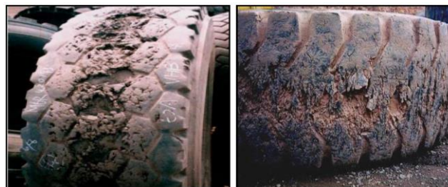
Figure 12. Haul Truck Tyre Tread Chunking.
