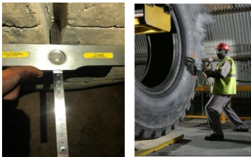
Figure 21. Haul Truck Tyre Being Repaired at NAM Site.
