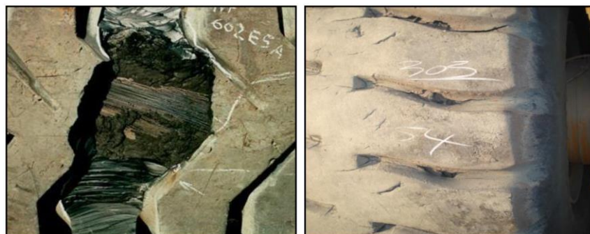
Figure 14. Haul Truck Tyre Separation.
