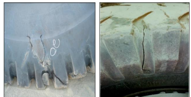
Figure 8. Haul Truck Tyre Shoulder Cut.
