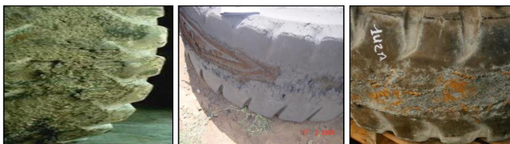
Figure 16. Tyre Worn Out.
