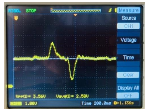
Figure 13. EOG signal from left to right eye movement.
