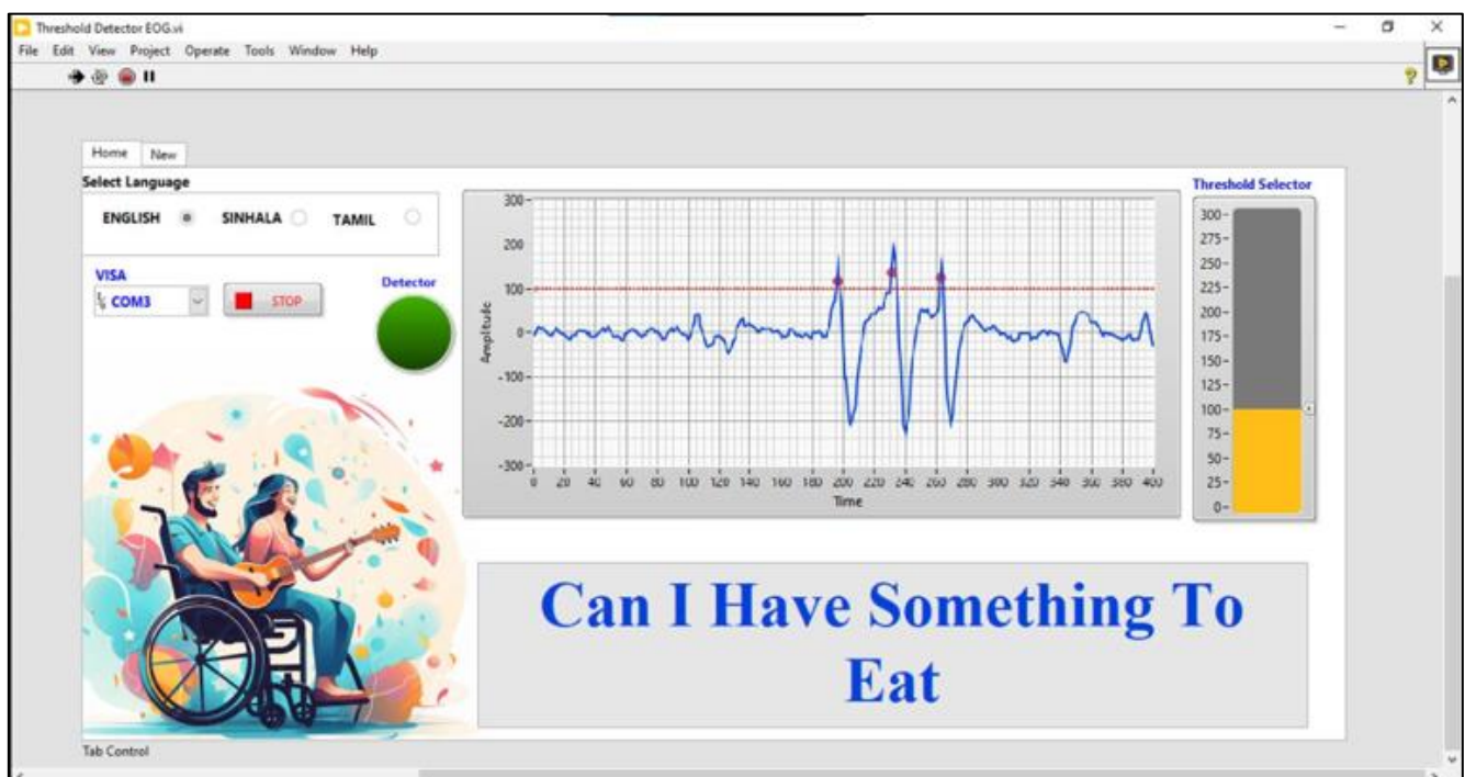
Figure 17. Virtual instrument output for three eye blinks.
