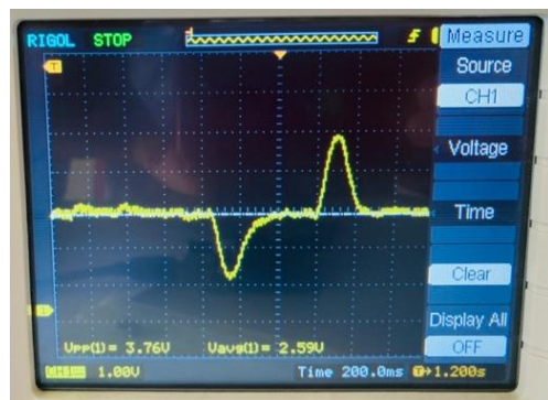
Figure 14. EOG signal from left to right eye movement.
