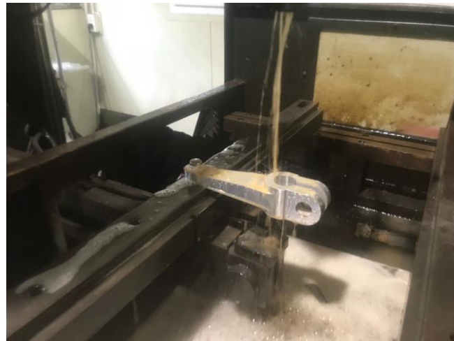
Figure 5. WEDM machining of the internal slot and keyed-bore features of the clamp-type linkage arm.
