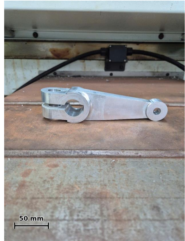
Figure 6. Completed aluminum clamp-type linkage arm after CNC milling and WEDM. The 50 mm reference scale was calibrated from the 120 mm center distance specified in Figure 2.
