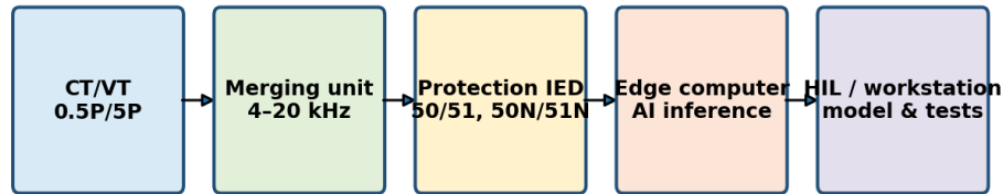
Figure 2. Measurement, IED, edge-computing, and HIL verification equipment chain.
