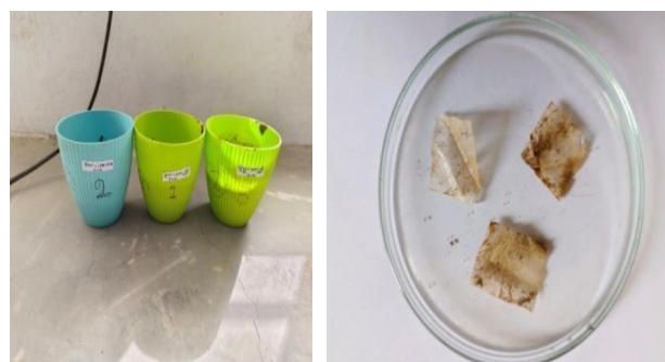
Figure 6. Experimental setup of the pot study showing LDPE strips incubated with Bacillus rugosus RB3 at 28\text{--}30^\circ\text{C} for 90 days to evaluate LDPE biodegradation efficiency.
