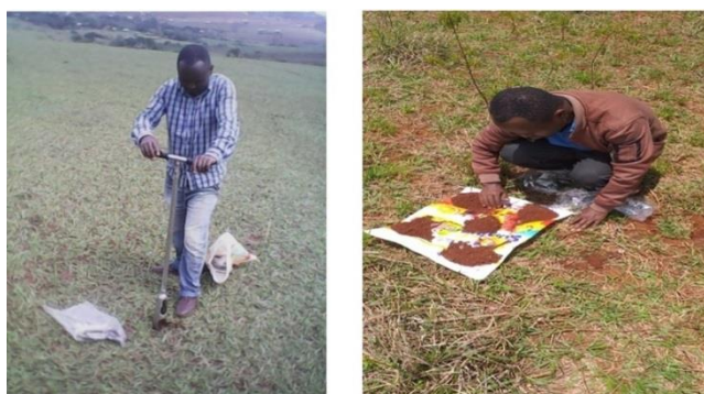
Figure 2. Soil sample collecting process.
