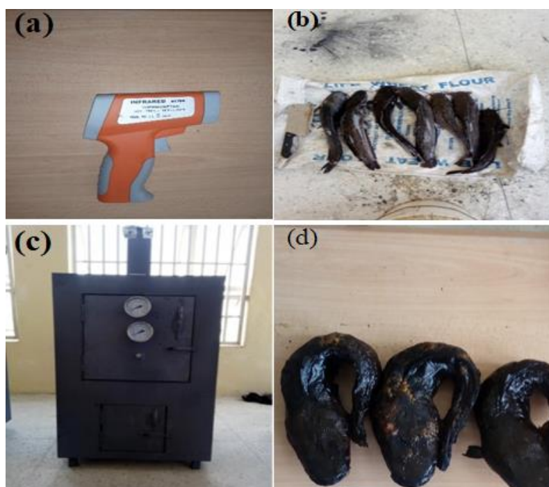
Figure 1. Experimental materials and fish smoking kiln: (a) Digital infrared thermometer used for temperature measurement, (b) fresh fish samples before smoking operation, (c) fabricated multi-chamber fish smoking kiln, and (d) smoked fish samples after drying and smoking process.
