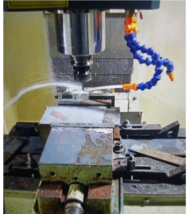
Figure 10. Actual machining of the lug-type pneumatic-cylinder base.
