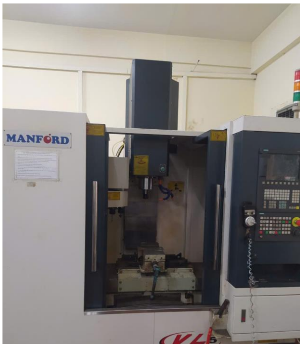
Figure 8. Manford CNC milling machine used for the workshop implementation.
