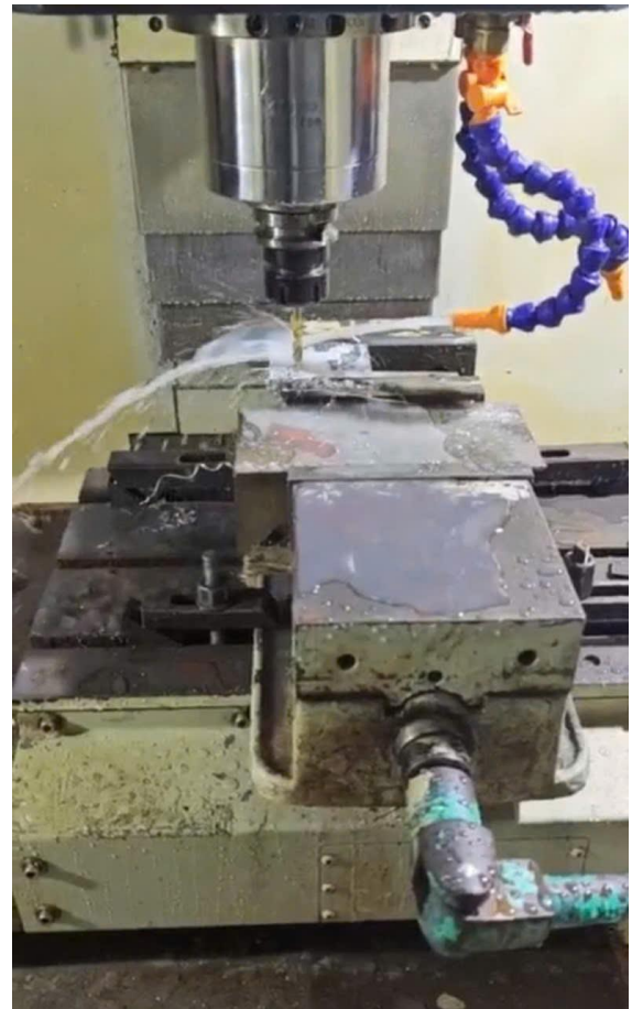
Figure 9. Actual machining of the plate-type pneumatic-cylinder base.
