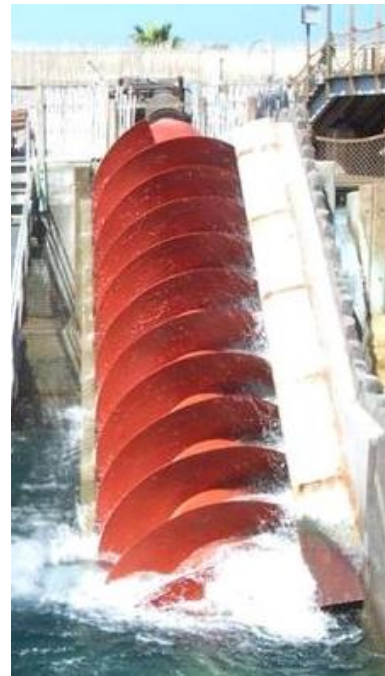
a) evolvent helicoid (Archimedes Screw)
