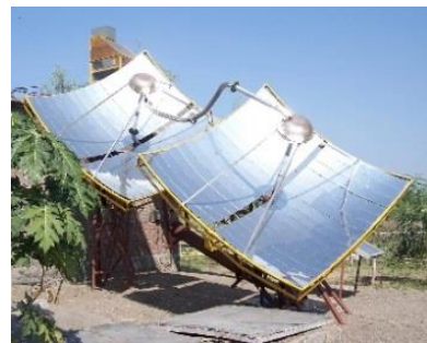
b) surface of translation of a parabola over another parabola (the parabolic sun concentrator)
