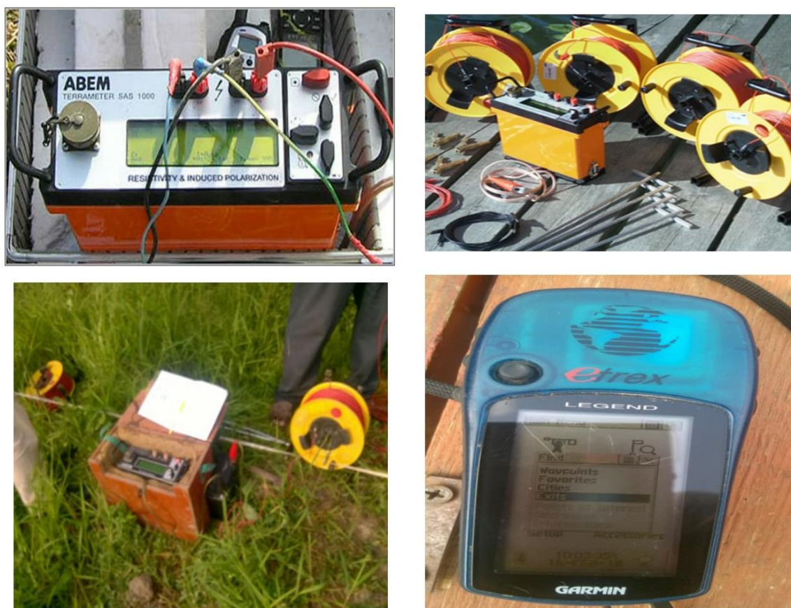
Figure 5. Abem Terrameter and accessories (Abem Terrameter (SAS 1000), Garmin etrex GPS) used in the study.
