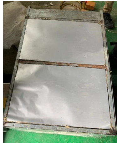
Figure 4. Oven insulation.
