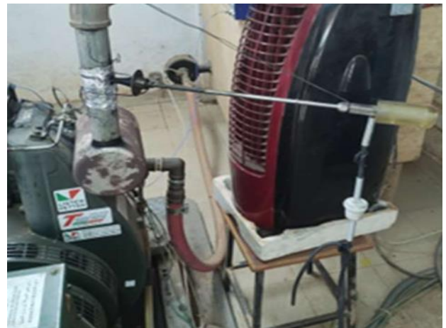
Figure 4. Experimental setup of the TESTO 350 gas analyzer probe.
