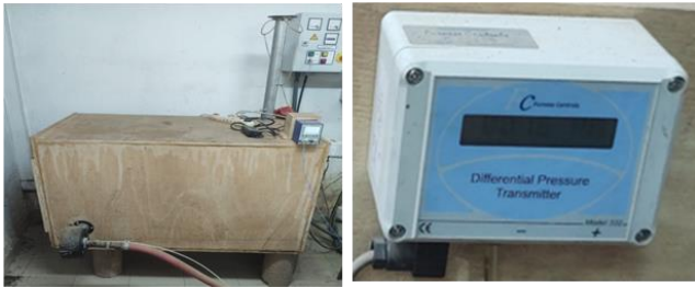
Figure 2. Air flow measurement system: The air chamber is on the left and the sensor is on the right.
