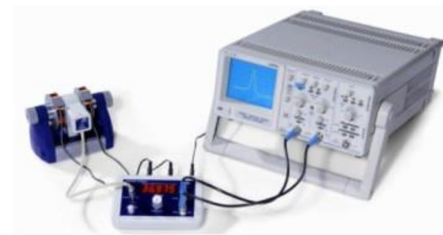
Figure 1. Experimental set up of Electron spin resonance Experiment.
