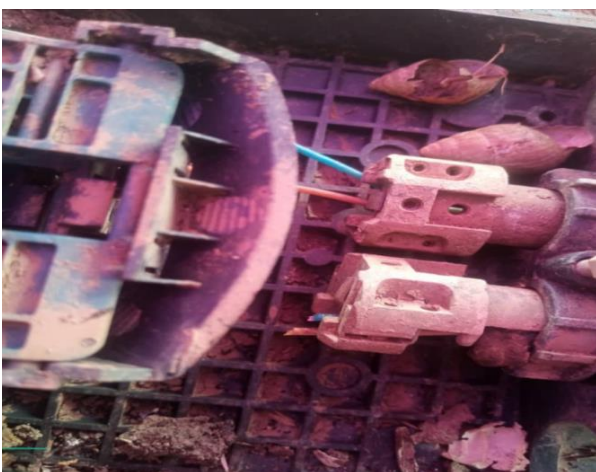
Figure 12. Optic fibre cable buffer eaten by rodents along Abuja Airport Highway Road.
