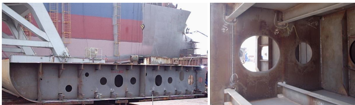
Figure 1. Cutouts in the ship structure.
