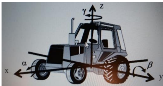
Figure 4. Tractor vibrations in relation to measurement points coordinate system ( X , Y , Z ) [3].
