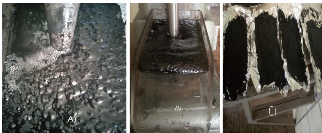
Figure 5. Froth flotation procedure and the resulting coal particles: (A) after adding the collector, (B) after adding the frother, (C) filtered concentrate.
