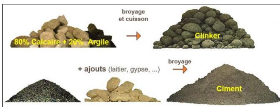
Figure 11. The main stages of cement manufacturing [82].
