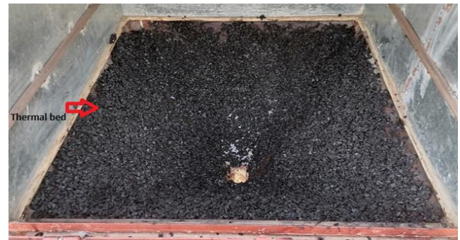
Figure 2. Thermal bed inside the solar dryer.
