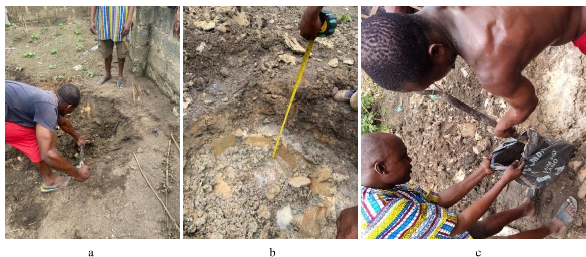
Figure 2. Processes in the sample collection: a, clearing and removing topsoil to reach desired depth b, measuring depth reached c, bagging of samples.
