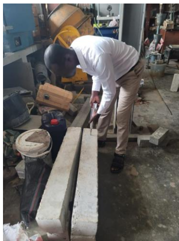
Figure 7. Rebound hammer test on concrete beam before flexural test.
