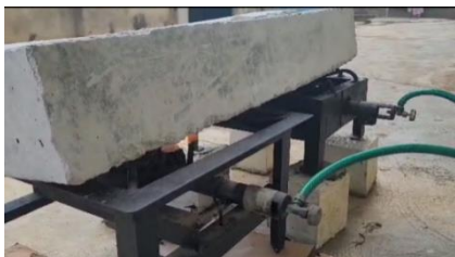
Figure 6. Image Showing Concrete Beam Heated to 600°C For 2 Hours Using an Open Fire.
