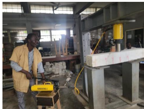
Figure 8. Beam Sample Undergoing Flexural Testing.
