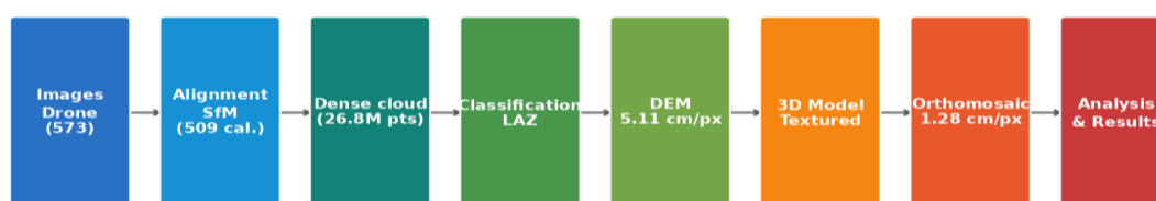
Figure 3. Complete photogrammetric processing pipeline, from raw images to final products.
