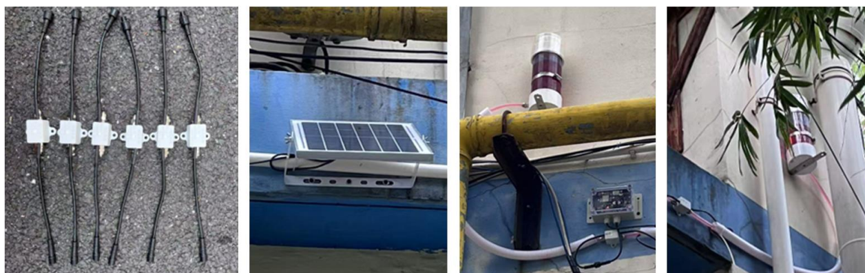
Figure 14. The static level sensor and field installation diagram.
