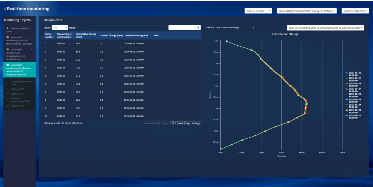
Figure 5. The automatic inclinometer monitoring data interface.
