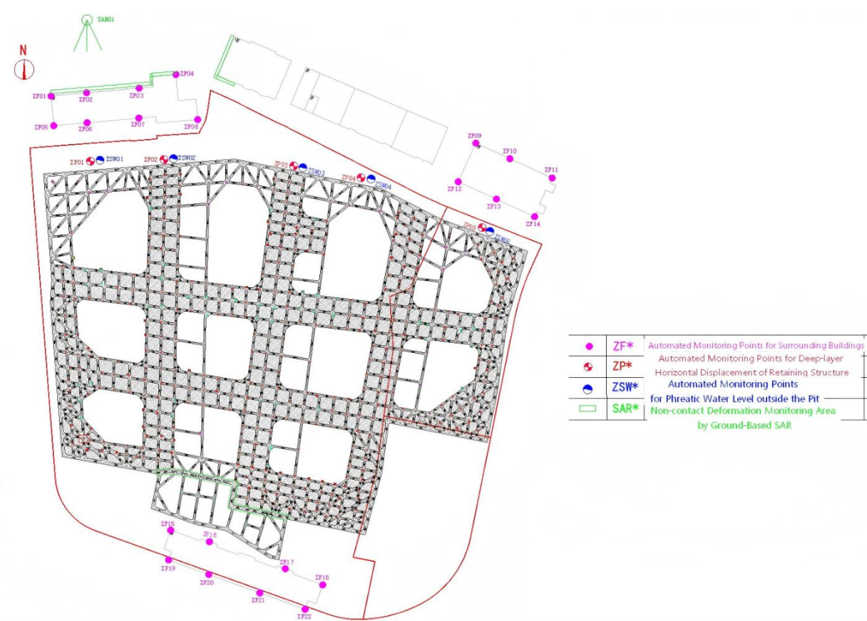
Figure 9. The layout of automatic monitoring points for a deep foundation pit project in Shanghai.
