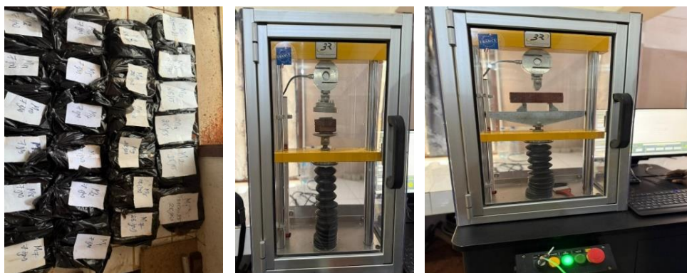
(d): sealing of the specimens in plastic bags before curing to avoid moisture variations (e): unconfined compression test (f): flexural tensile strength
