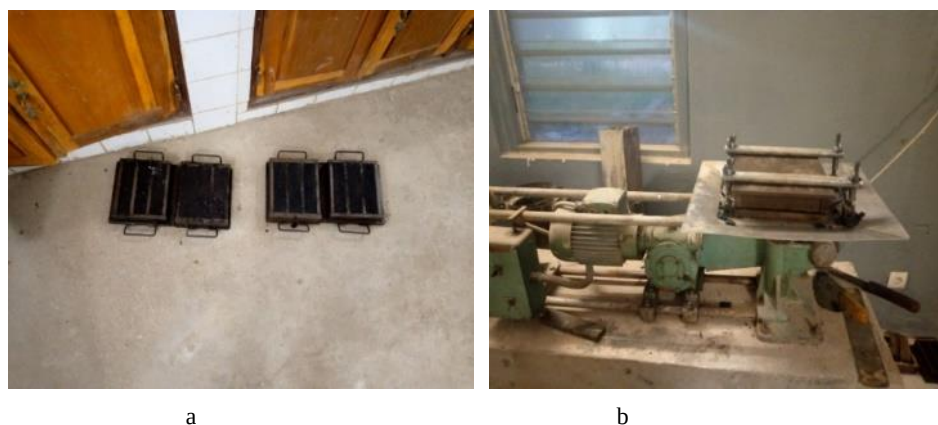
Figure 2. a. Casting into a mould b. Compacting of the material in the mould.
