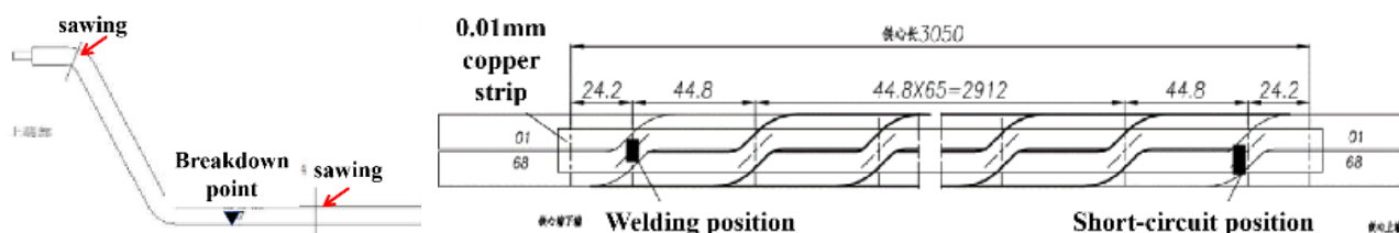
Figure 6. Internal shielding process diagram.
