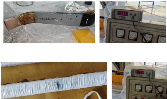
Figure 5. Stator bar transient breakdown test.
