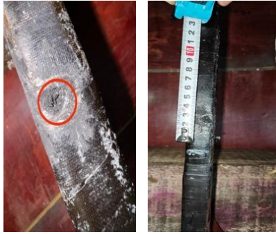
Figure 2. Breakdown point of stator bar.
