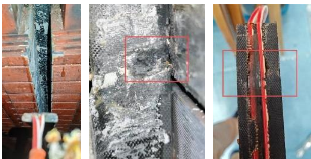
Figure 4. Location of the burning point of the side temperature measuring pad between layers.
