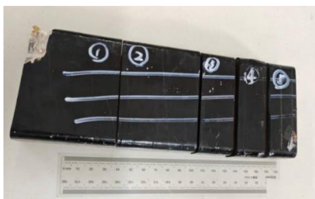
Figure 7. Stator bar segment marking.
