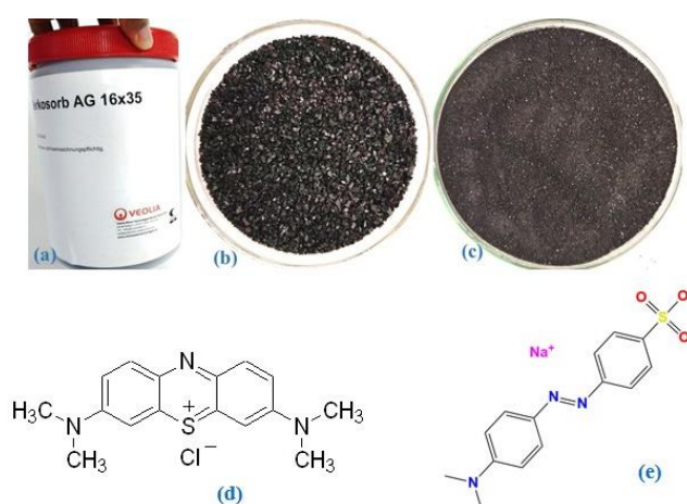
Figure 1. Container of the activated carbon supplied by the manufacturer (a), granular form of the activated carbon (b), powdered form of the activated carbon (c) and methylene blue (d) and methyl orange (e) molecular structure.
