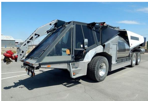
Figure 21. Colet vehicles with firefighting arm - lowest position.
