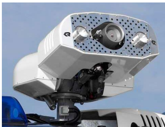
Figure 14. Modern European water and foam turrets Rosenbauer RM 60 with non-aspirated nozzle.
