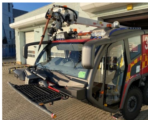
Figure 31. The fold-out platform on the WISS Felix II car (2012).
