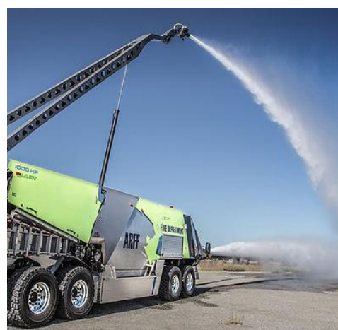
Figure 20. Colet vehicles with firefighting arm - highest position.
