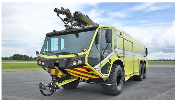
Figure 23. American designs of short drop arms with turrets E-One.
