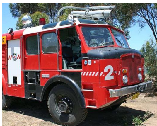
Figure 32. The simplest solution - a Thornycroft Nubian 6X6 (1968) with a bonnet adapted to the function of a support platform [28].
