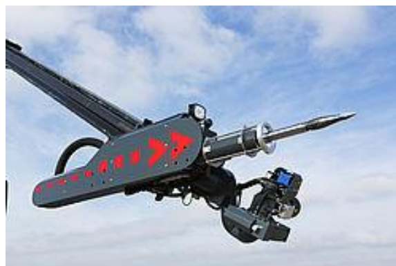
Figure 25. Rosenbauer punch with an additional forcing actuator.
