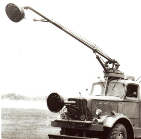
Figure 18. The prototype, the firefighting arm of the CC 150 Cardox car on a Mack chassis (1947) [2].
