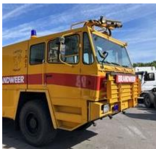
Figure 29. A simple platform on a MAC 6 Saval-Kronenburg (2001).
