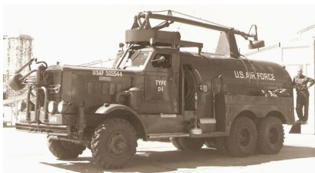
Figure 5. C 150 Cardox vehicle on Sterling chassis year of manufacture 1943 [2].
