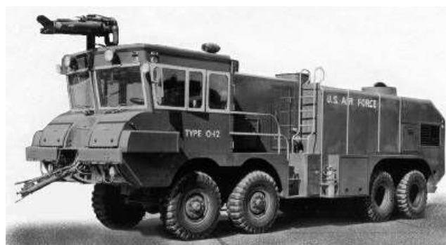
Figure 33. Prototype vehicle O-12 on a special 8x8 chassis, like the earlier O-10 and O-11 were the inspiration for many US manufacturers [13].
