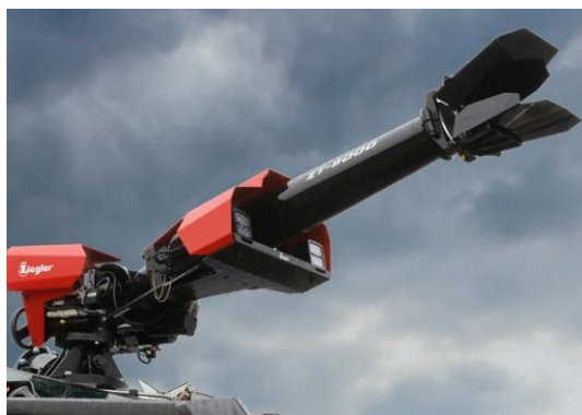
Figure 13. Modern European water and foam turrets Ziegler Z 8000 with classic aspirated nozzle.
