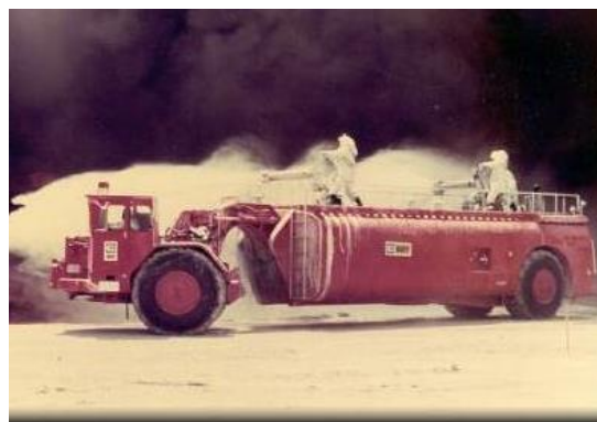
Figure 37. An experimental vehicle probably based on the M 520 Goer.
