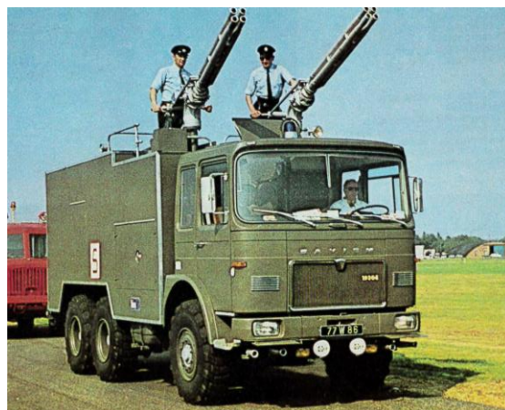
Figure 42. Airport rescue and firefighting vehicles without an auto-pump, French Birocarbo 5500.
