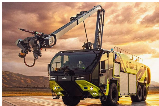
Figure 19. The modern version of the HRET arm on the Oshkosh Strker 6x6 car (2023).
