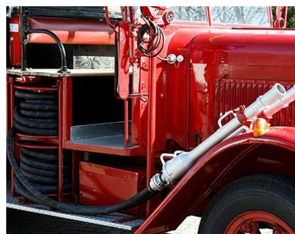
Figure 7 Two-line rapid attack device on a Kfz.343 Henschel car (1936) [8].
