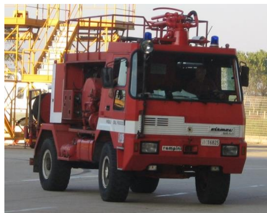
Figure 41. Airport rescue and firefighting vehicles without an auto-pump, Italian Sirmac Rampini 524D 4x4 Rambo [31].
