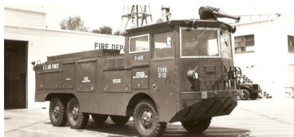
Figure 12. Type 0-10 fire and rescue truck (1950) probably the first mass-produced vehicle with a roof-mounted turret [13].
