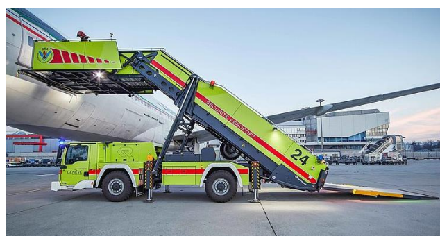
Figure 28. Modern staircase on a vehicle chassis, adapted for rescue purposes by Rosenbauer.
