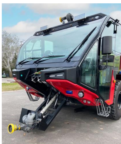
Figure 22. American designs of short drop arms with turrets, by Oskosh.
