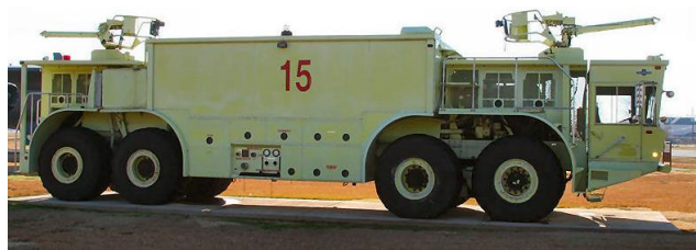
Figure 15. One of the 80 Oshkosh P-15 fire and rescue vehicles produced in 1978 [13].
