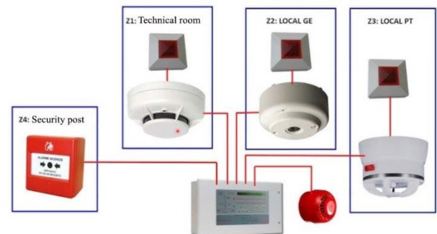
Figure 3. Automatic fire detector system [24].
