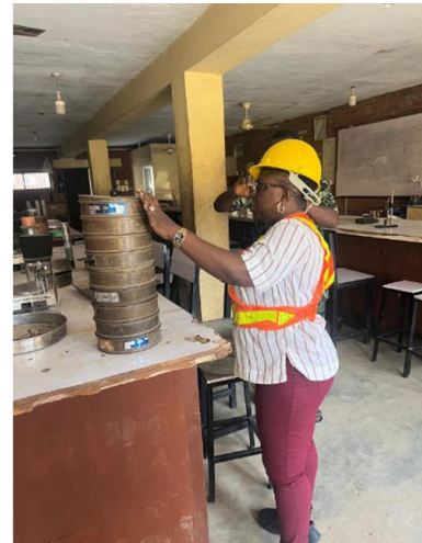
Figure 5. Sieve Analysis Process in the Laboratory.
