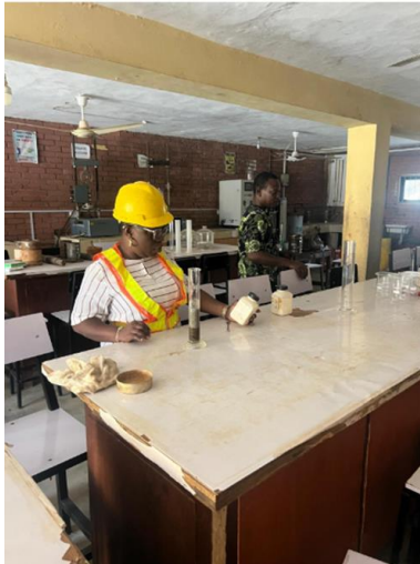
Figure 4. Water absorption and Specific Gravity Process in the Laboratory.
