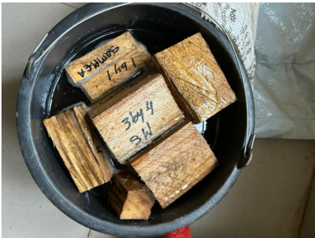
Figure 6. Soaked Timber Samples.
