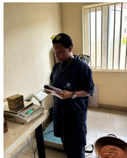
Figure 7. Weighing Timber Samples.
