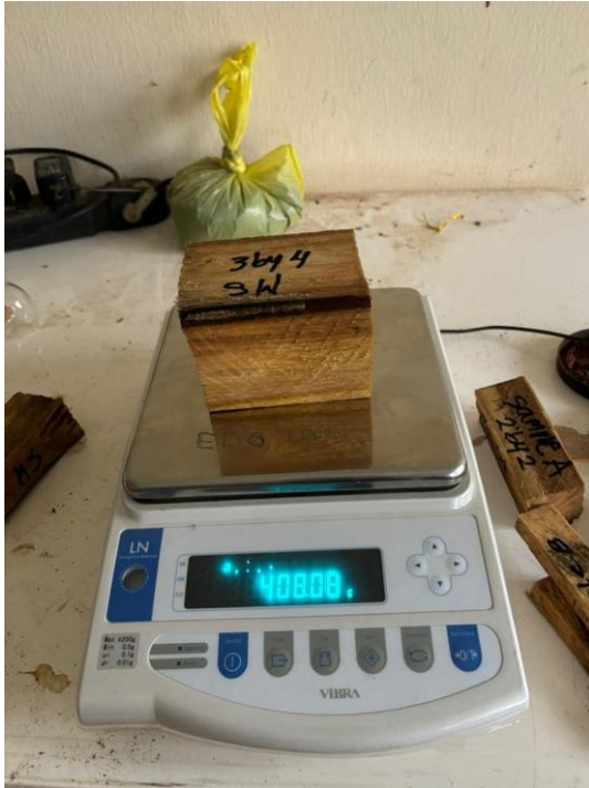
Figure 4. Test sample being weighed.
