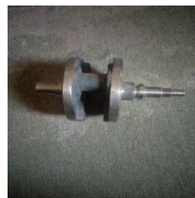
Figure 2. ADI Crankshaft with In-gates.
