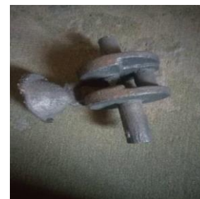
Figure 1. ADI Crankshaft without In-gates.
