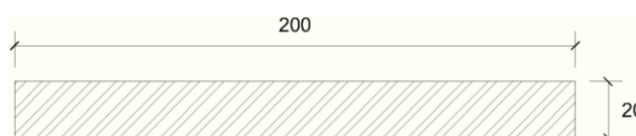
Figure 10. Typical Steel plate size for tensile test (dimensions in mm).
