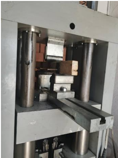
Figure 14. Setup of Timber-Plate beam connected with Steel for UTM flexural Test.
