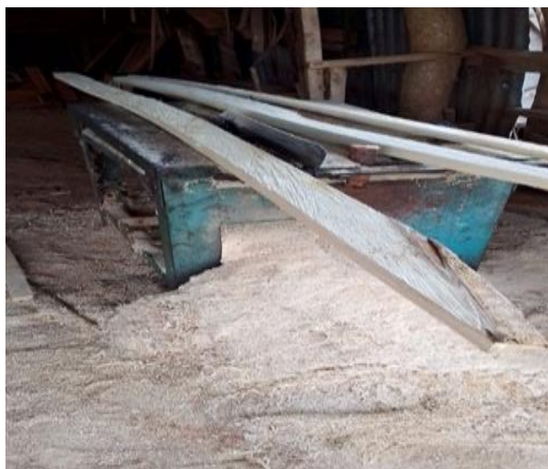
Figure 2. Sawing of Opepe Timber.
