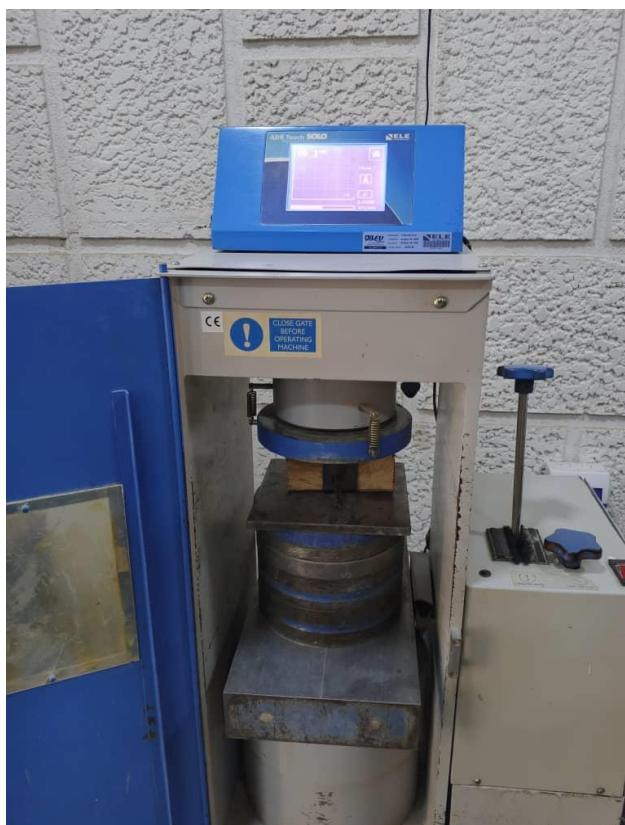
Figure 8. Compression Test for Opepe Timber in UTM.
