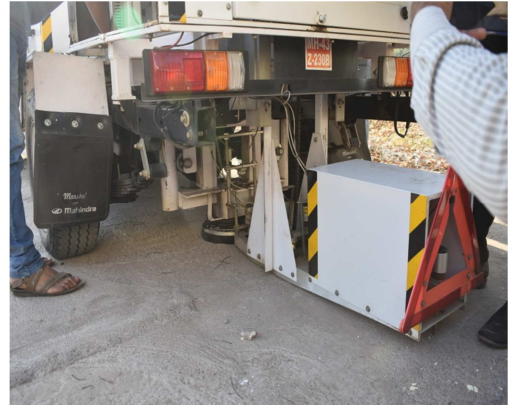
Figure 1. Falling Weight Deflectometer Machine Testing on the pavement.
