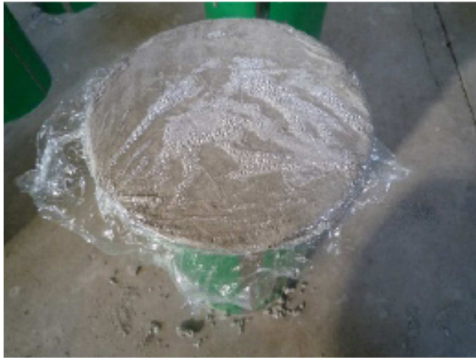
Figure 1. Sealed curing (AN).
