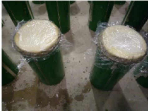
Figure 2. Wet curing (AA).
