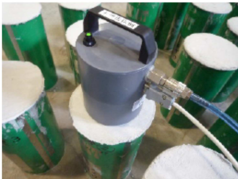
Figure 4. View of air permeability test.
