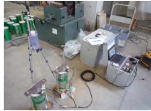
Figure 5. View of water absorption test.
