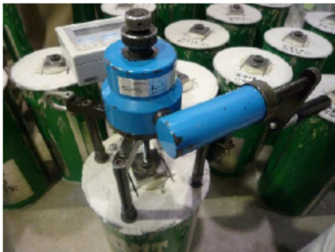
Figure 3. View of surface tensile test.
