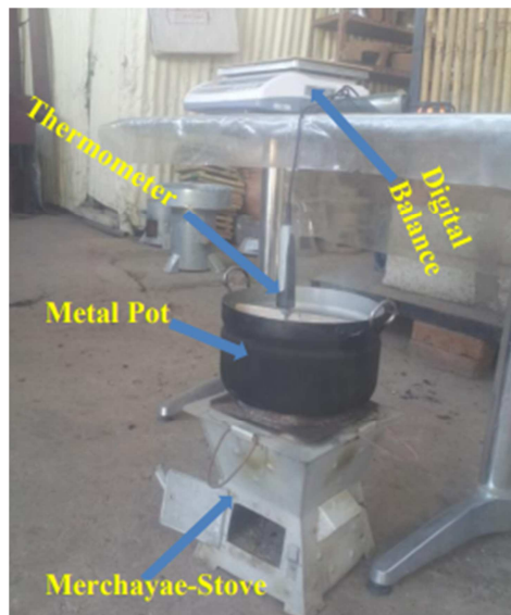
Figure 25. Combustion and water boiling capacity test.
