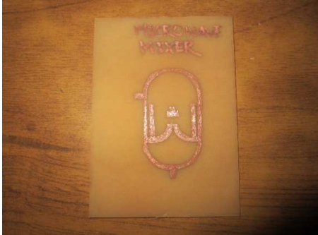
Figure 11. Fabricated Mixer layout on copper board.
