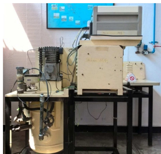
Figure 2. PLINT, the air compressor system.
