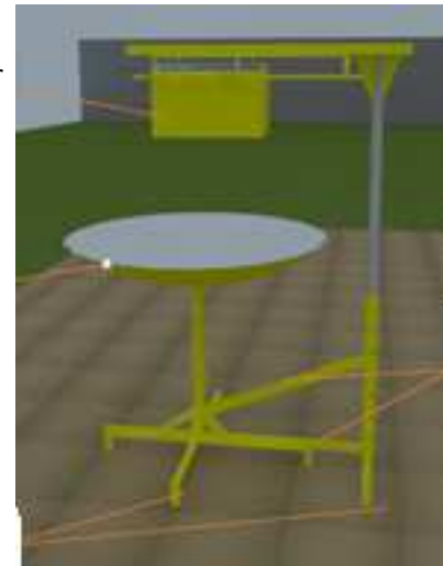
Figure 5. Modelled view of the solar cooker in 3D.
