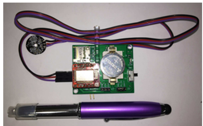
Figure 10. Wearable Gauge (37mm x 50mm).
