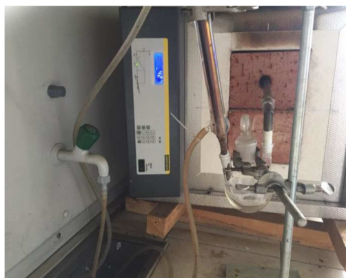
Figure 3. Furnace and distillation chamber setup.
