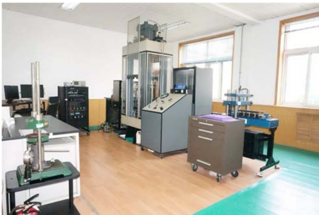
Figure 4. Test mechanics for Three axis stress testing of rock.
